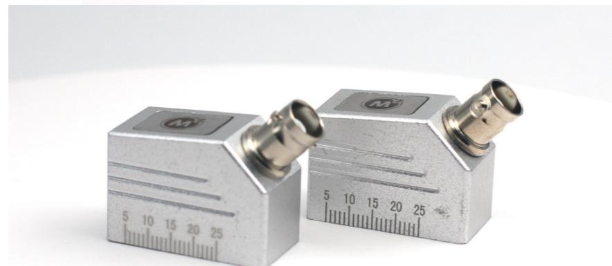
The angular beam probe is a single crystal probe used with a wedge, which can be replaced to emit refracted shear or longitudinal waves into the workpiece under test.
